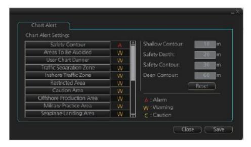
Click a letter indication to select the type of alert, warning or caution, to receive for the fiven chart object. [Safety Contours] is fixed to "A" (Alarm).
